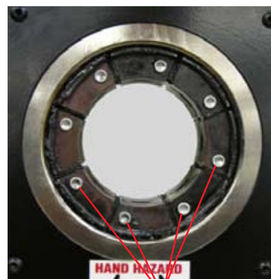
Grease Fitting Holes
