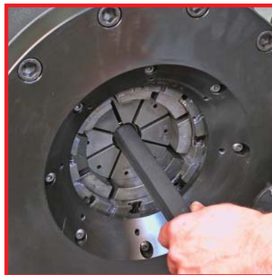
Position the fitting against the Coupling Stop and actuate the crimper in the normal manner.
