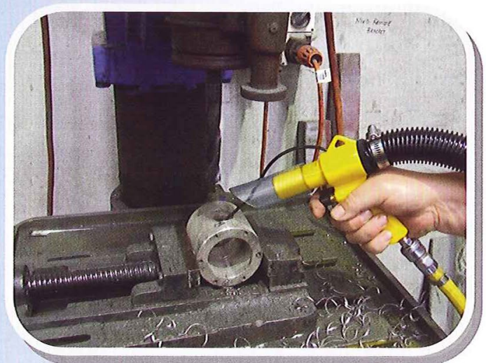
Clearing metal pieces out of drilled holes.
